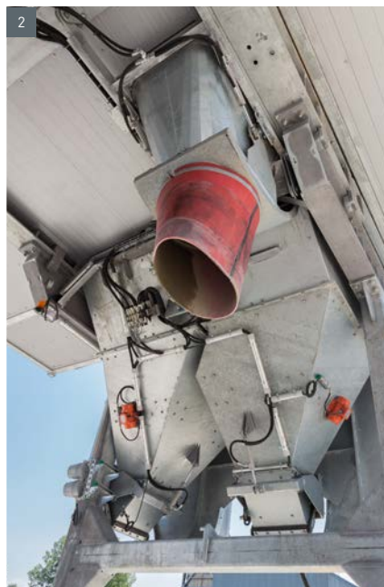
1. Schwenktrichter / Swivel funnel ■ 2. Betonabgabe Betonpumpe / Concrete discharge for concrete pump ■ 3. Betonabgabe Krankübel / Concrete discharge for crane bucket
