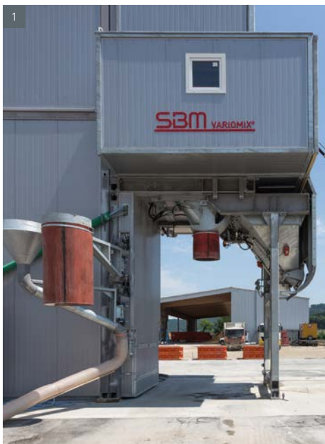
1. Schwenktrichter / Swivel funnel ■ 2. Betonabgabe Betonpumpe / Concrete discharge for concrete pump ■ 3. Betonabgabe Krankübel / Concrete discharge for crane bucket
